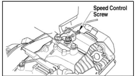
The maximum speed of the snowmobile can be reduced by adjusting the speed control screw.
