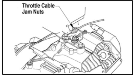
2. Pull all slack from the throttle cable wire and exert slight tension on the wire.
